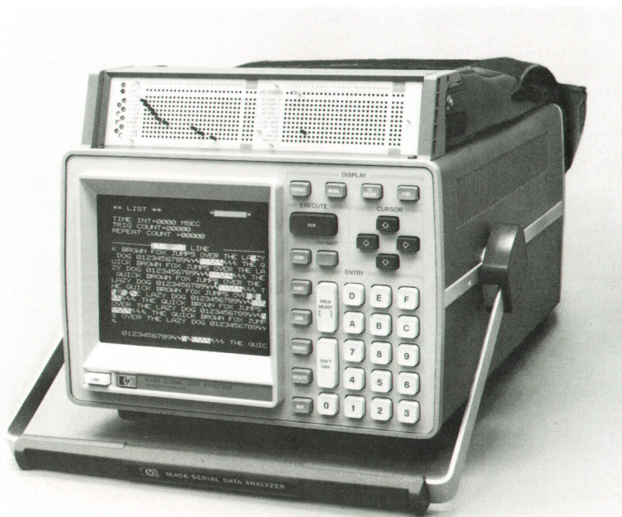
Fig. 1. Model 1640A Serial Data Analyzer is a portable logic analyzer tailored for the troubleshooting and analysis of systems tied together by serial data communications buses. Its capability for both monitoring and simulation enables it to analyze a whole spectrum of problems associated with malfunctioning systems that use communications buses.
